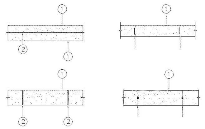
1. **Precast Autoclaved Aerated Concrete Wall Panels** — Min 4 in. thick by max 2 ft wide panels for 4 hr nonbearing wall rating. Min 6 in. thick by max 2 ft wide panels for 4 hr bearing wall rating. Panels installed either horizontally or vertically. Panels mechanically attached to the concrete floor and ceiling.
